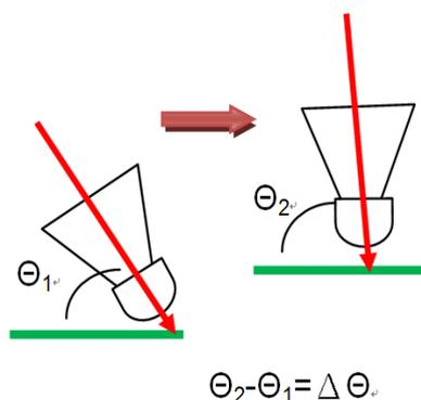
Figure 3: Shuttlecock tumbling angle definition.
