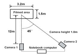
Figure 1: Measurement setup.
