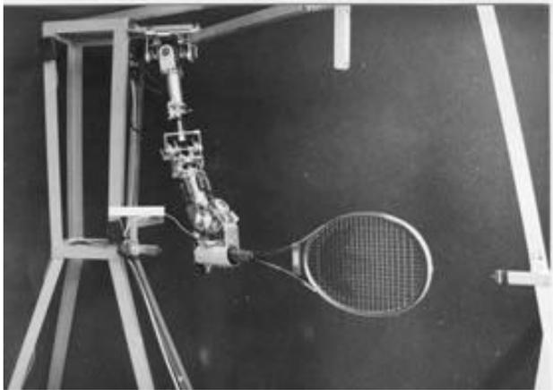
**Fig. 11:** *The manusimulator, a mechano-electronic device for testing objectively the biodynamical properties of tennis rackets. Shown are the artificial arm mounted on its base, the test racket held by the simulator hand, and the three lasers for precise position adjustment of the racket (From Hatze, 1992)*
