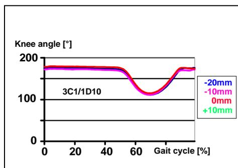
Figure 3: Knee angle depending on prosthetic alignment (see Fig. 4)
