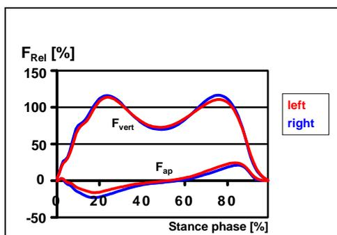
Figure 5: Ground reaction force during stance phase (in case of M.S.)
