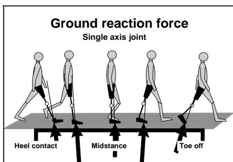
Figure 2: Ground reaction force during prosthetic stance phase in case of single axis knee joints
