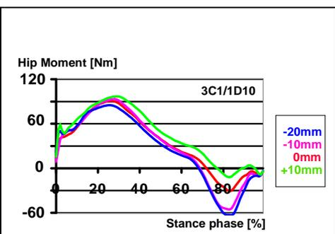
Figure 4: External moment of prosthetic knee joint and hip joint depending on prosthetic knee joint position (-20 to +10 mm in relation to normal fitting alignment)
