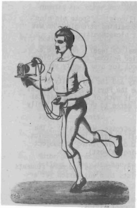
Figure 1. Man in action carrying a device to record pressure vs. ground and vertical movement of the head. (Marey, E.J., La Machine Animal, Felix Alcan, Paris, 1886)
