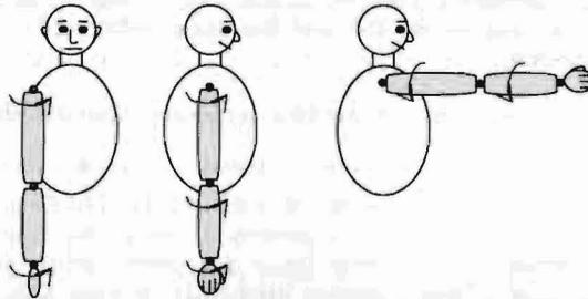
**Figure 2 Generalized coordinates  $q_r$  describe the position of upper limb.**
