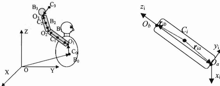
Figure 1 Kinetic model of human upper limb.
