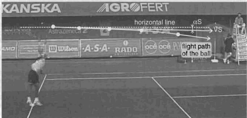
Figure 2 Kinematic analysis of the flight path of the ball after serve and measured variables.
