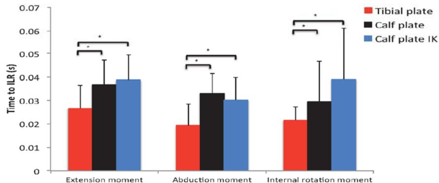
Figure 3. Time of peak ILR from the instant of landing (first 50 ms). Moments derived from the tibial plate data have significantly earlier peak slope of moment.
