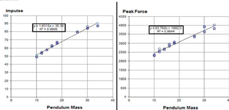
**Figure 2. Linear regression of dependent variables and pendulum masses.**
