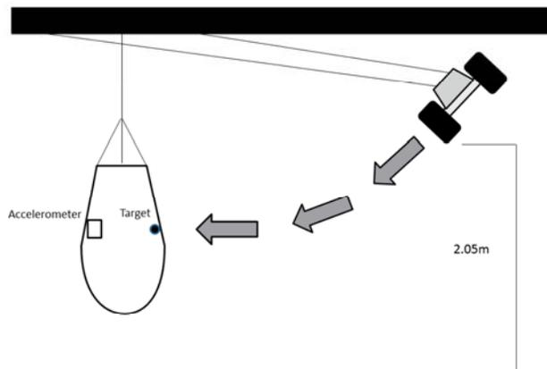
**Figure 1. A non-scale diagramme of the experimental set up.**
