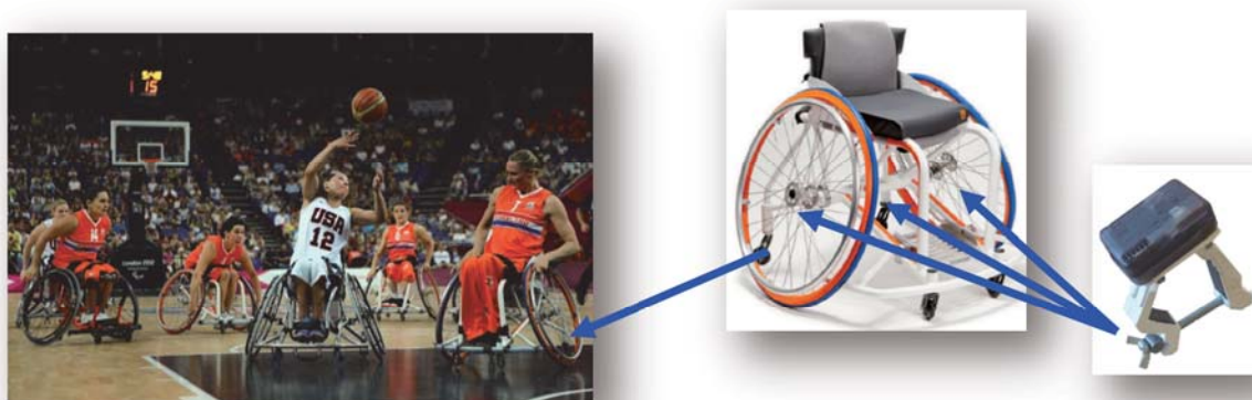
Figure 1: Measurement setup, with IMUs at on wheels and frame measured during a match.
