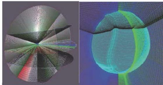
Figure 1 Grid system ( $327 \times 181 \times 101$ )
