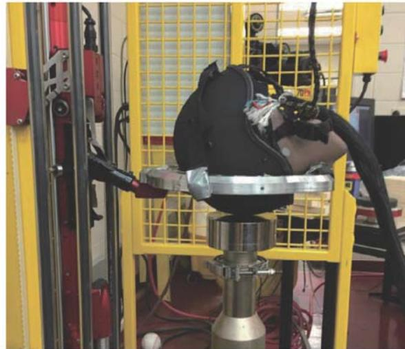
Figure 1: Monorail drop system used for unrestrained drops
