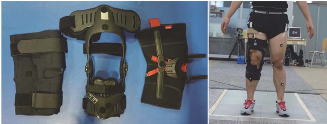
Fig. 1 Three kinds of commercialized knee brace (neo, CTI and patella-pro in order) and right figure shows marker setting in wearing knee brace.
