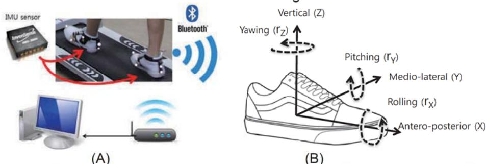
**Figure 1: (A) Shoe-type IMU sensor with reflective markers, (B) Directional definitions of six directional kinematic data for normal gait**
