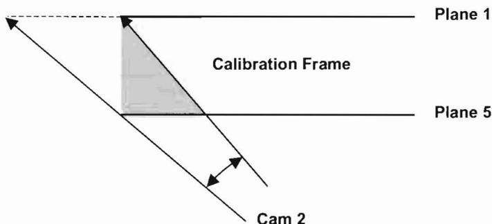
**Figure 2.** Extrapolation on plane 1 in camera 2 (overhead view). Control points in the gray area will be projected to outside of plane 1 (broken line) in the double-plane method although they are within the control volume.
