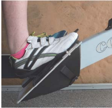
Figure 1 – Traditional foot-stretcher (raised heel at catch).
