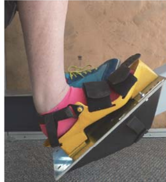
Figure 2 – Modified foot-stretcher (wedge at toes and heel).
