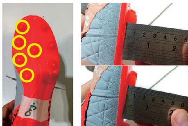
Figure 1: Medial-side part (left), original stud (right top), modified stud (right bottom)
