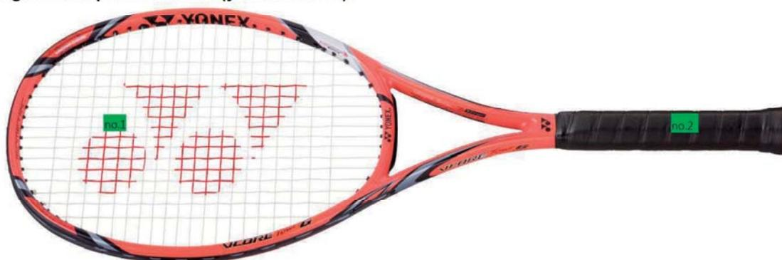
Figure 2: Location of accelerometers (green rectangles).
