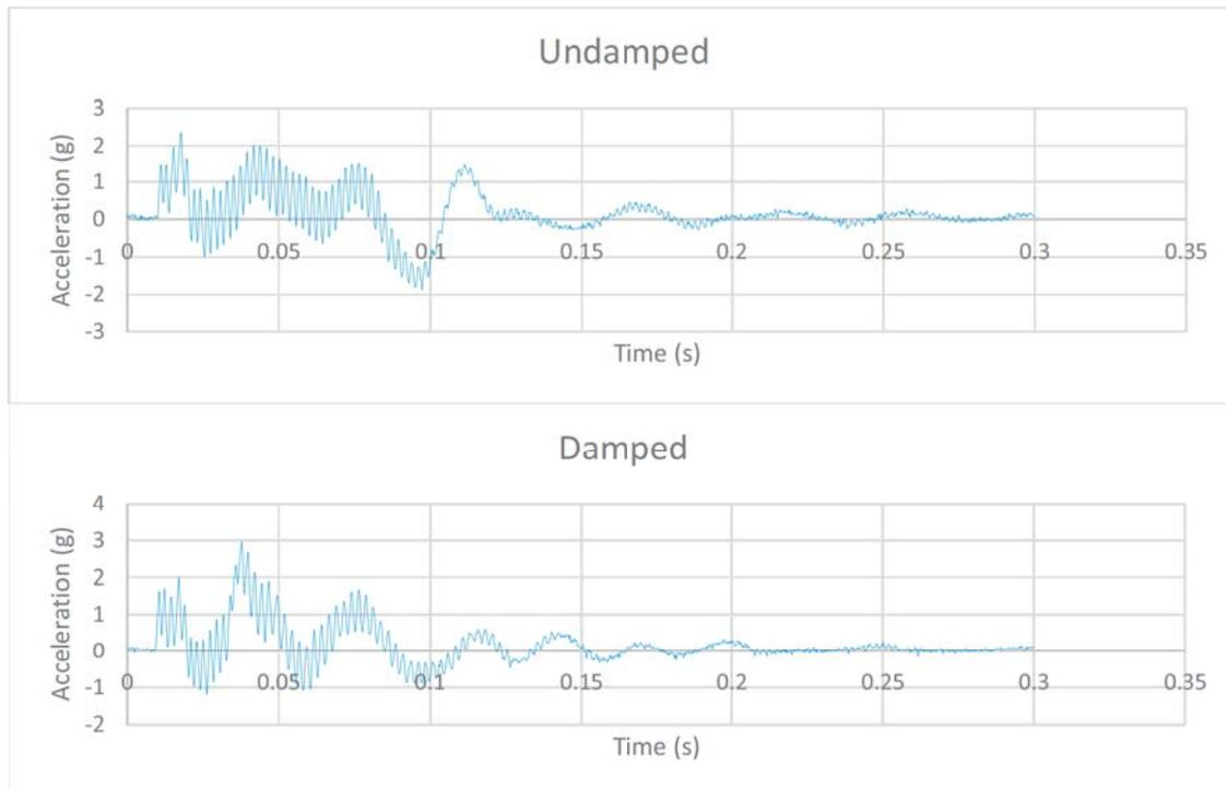
**Figure 3: Acceleration data of accelerometer no.1 with/without the damper.**
