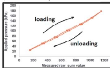
Figure 3: Grip sensor under loading and unloading pressure in area B.
