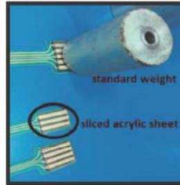
Figure 2: Illustration of loading with standard weight and acrylic sheets.
