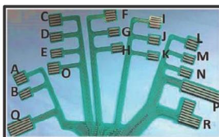
Figure 1: The real loading areas in 4256E grip sensor. (Area B,D,E,G,H,J,K,M,N are 1.92 cm<sup>2</sup> ; A,C,F,I,L,O are 2.56cm<sup>2</sup> ; Q is 7.20 cm<sup>2</sup> ; R is 8.32 cm<sup>2</sup> and P is 9.44 cm<sup>2</sup>)
