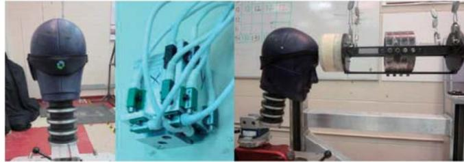
**Figure 1: Triax Smart Impact Monitor positioning (left), headform accelerometer array (middle), and pendulum impacting system and NOCSAE headform (right)**
