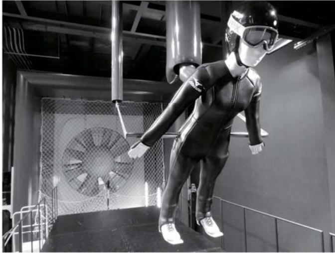
Figure 1 A full-scale model of a female ski jumper in the wind tunnel.
