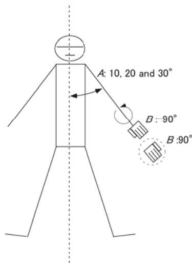
Figure 3 Definition of the Arm ( $A$ ) and the hand ( $B$ ) positions of the ski jumper model in the wind tunnel test.
