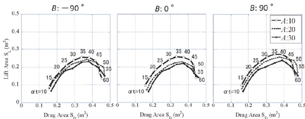
Figure 4 The effects of shoulder abduction ( $A$ ) on the lift and drag area in each orientations of the hands ( $B$ ) with attack angle of trunk ( $\alpha t$ ).
