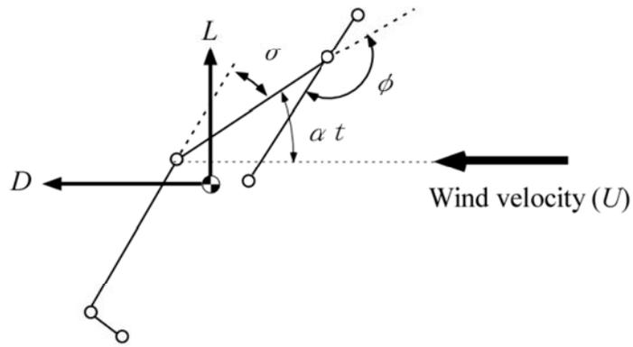
Figure 2 Aerodynamic parameters (lift ( $L$ ) and drag ( $D$ ), and flight positions ( $\alpha t$ ,  $\sigma$  and  $\phi$ ) of the ski jumper model in the wind tunnel test.
