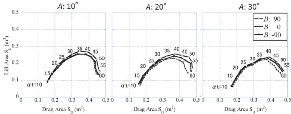
Figure 5 The effects orientation of hands ( $B$ : direction of palms) on the lift and drag area in each shoulder abduction condition ( $A$ ) with attack angle of trunk ( $\alpha_t$ ) .
