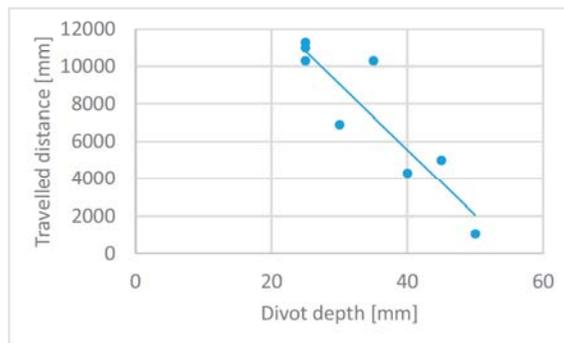
**Figure 5: (a) Travelled distance vs. divot**
