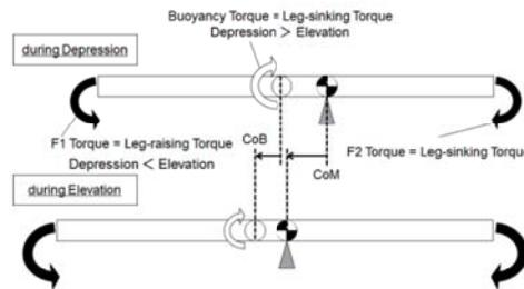
**Figure 5: Schematic view of the body torques change due to the change of the total length.**
