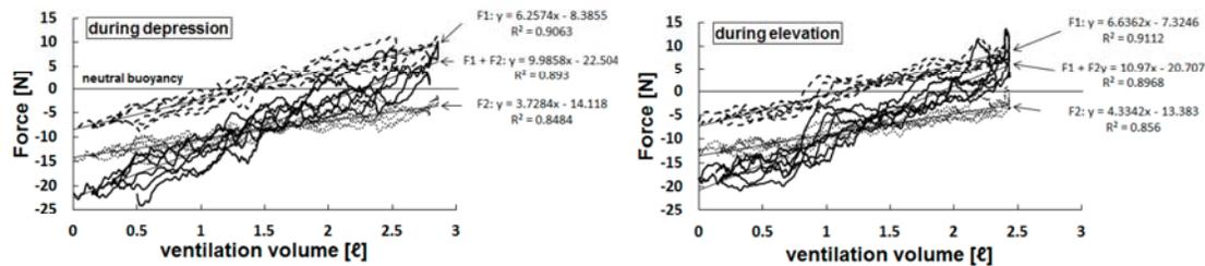
Figure 2: Change in buoyancy because of the change in ventilation volume.
