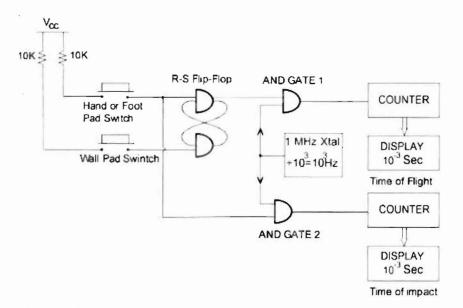
Figure 1 - Eedronic schematic for determination of initial ball velocity and the impact force.
