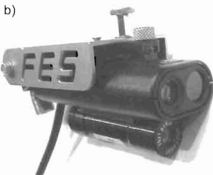
Figure 2. a) Functionality of the system b) Modified NOPTEL-ST-2000-system. The weight of the optical unit is 160g, dimensions: 100*40*100mm.
