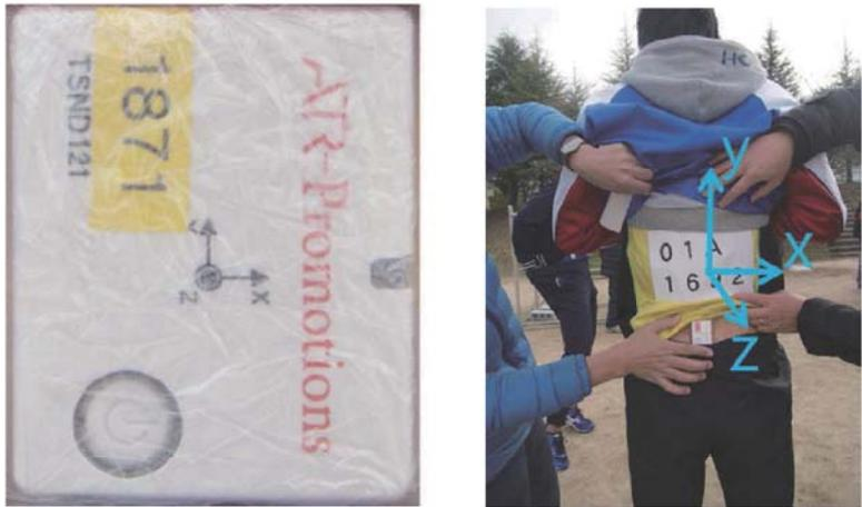
Figure 1: Sensor used for the experiment (Left), and how it was attached (Right)
