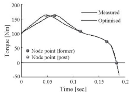
**Figure 2: Schematic view of the measured and optimised joint torques about the pivot hip flexion/extension axis.**
