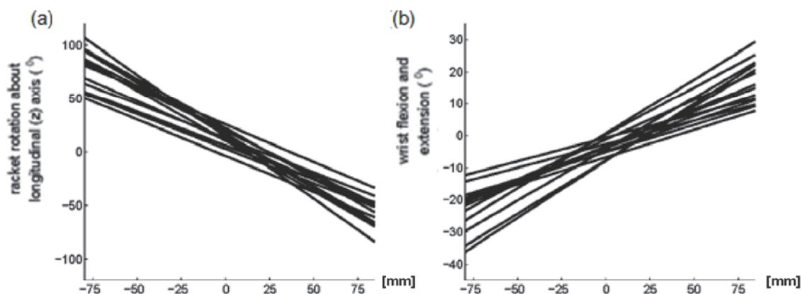
**Figure 1: The relationship between off-longitudinal axis impact locations and (a) racket rotation about the longitudinal axis, (b) wrist flexion / extension for all participants.**
