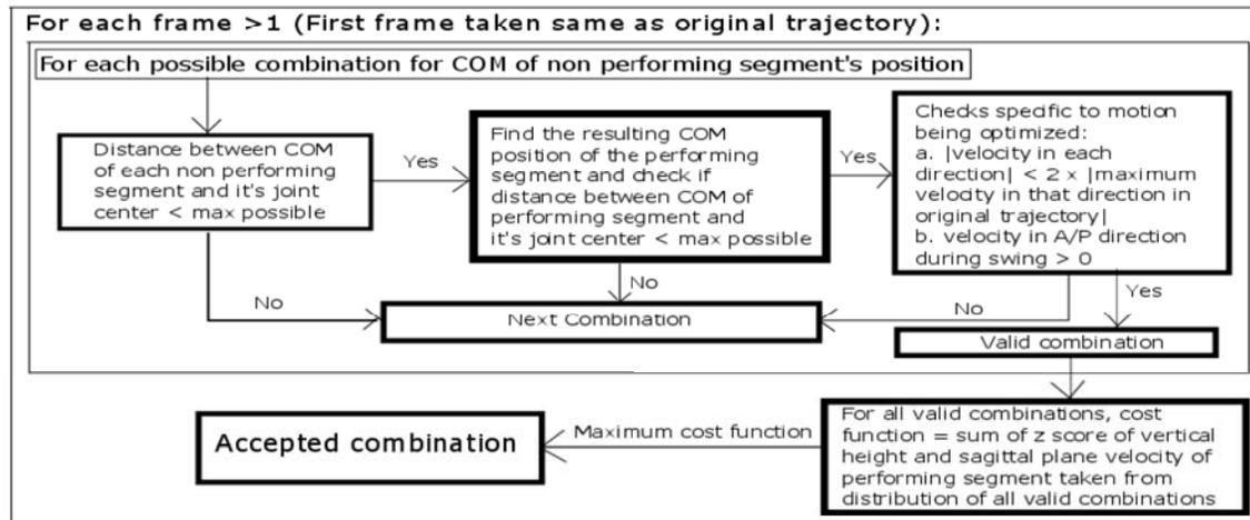
Figure 1: Flow chart of the optimizer
