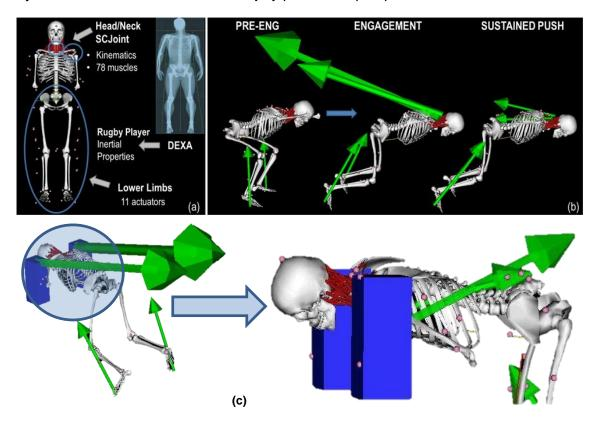
**Figure 1.** (a) The full body 'Rugby Model', specifically optimised for rugby activities dynamic analysis. (b) Full body motion and external load application of an individual player scrummaging, divided in the main three phases of a rugby scrum: preengagement, engagement and sustained push. (c) Inclusion of the scrum pads in the model in order to minimise experimental inaccuracies.
