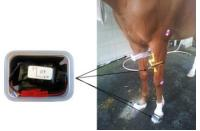
Figure 1: The sensor unit in the casing (left) and the four sensors mounted on forearm and hoof (right).
