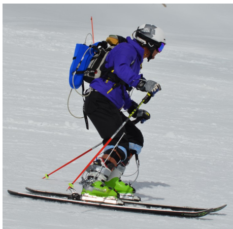
Figure 1: Instrumented skier with dynamometers, goniometer, DGPS and inertia sensors.
