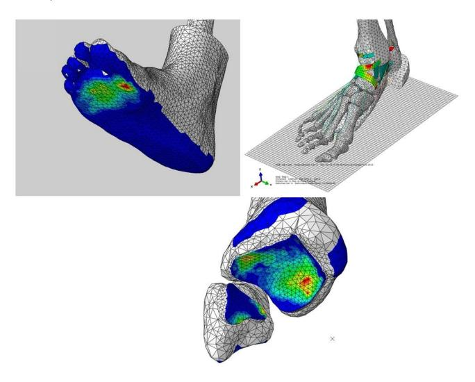
Figure 2: Examples of field data that can be extracted from the model, during a running cycle, foot contact pressure (top left, blue = 0 MPa, red = 0.5 MPa), in plane principal stress on the ligaments (top right, blue = 0 MPa, red = 60 MPa), tibia cartilage contact pressure (bottom, blue = 0 MPa, red = 13 MPa).
