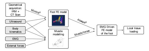
Figure 1: Complete process of model building, including the finite elements part and the tendon forces estimations.
