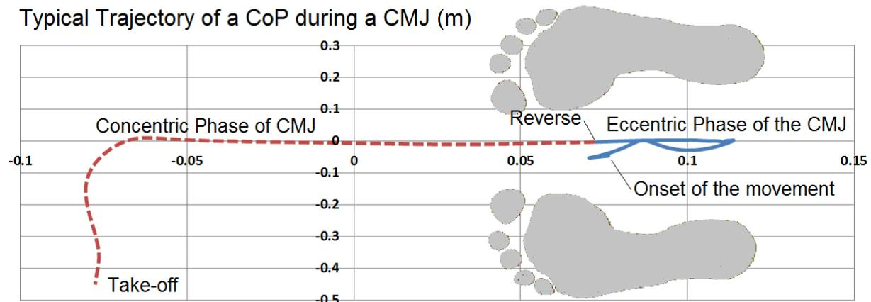
**Figure 1: Typical CoP trajectory during a CMJ, showing the initial position of the feet (not to scale) and its two phases. In this case, the subject took off asymmetrically, leaving the ground with his left toe.**
