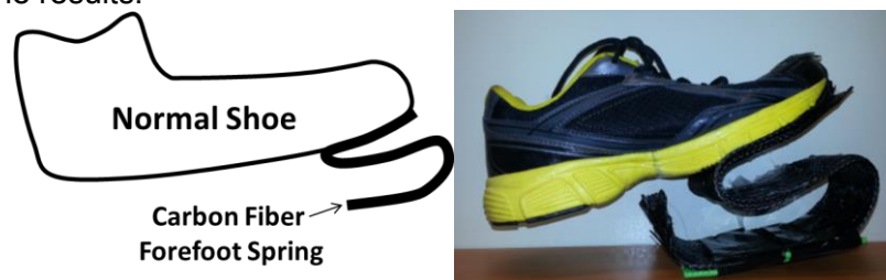
Figure 1: (Left) schematic of the forefoot-spring footwear and (Right) photograph of the forefoot-spring footwear.
