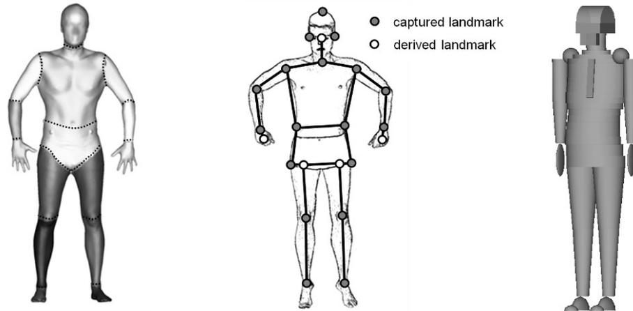
**Figure 1: Left: Segmentation of the subject with body scanner software AnthroScan (Human Solutions, 2005). Center: Reaction board model. Right: Geometric dynamic model.**
