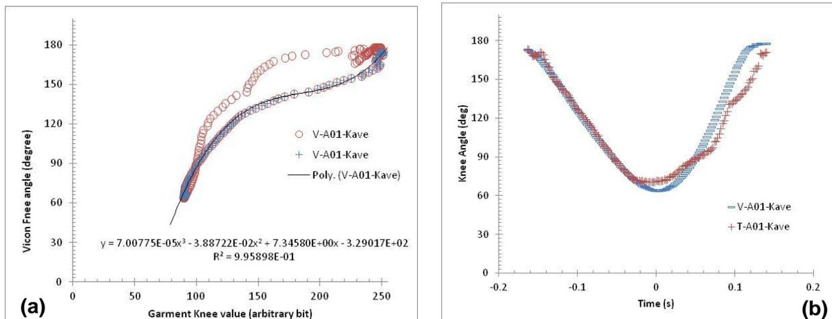
**Figure 4 (a) Garment Calibration using flexion component of movement and, (b) comparison of associated knee angle derived from sensor and Vicon analysis.**
