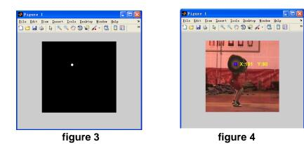
Using MATLAB image processing toolbox (IPT) to processed image spot analysis, find out the index point image center and rectangular to color piece for mark, intrturn to mark the image center coordinates.
