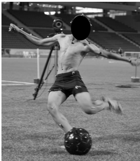
Figure 1: Player performing IK with the non-preferred leg - location of reflective markers on the ball and player shown.
