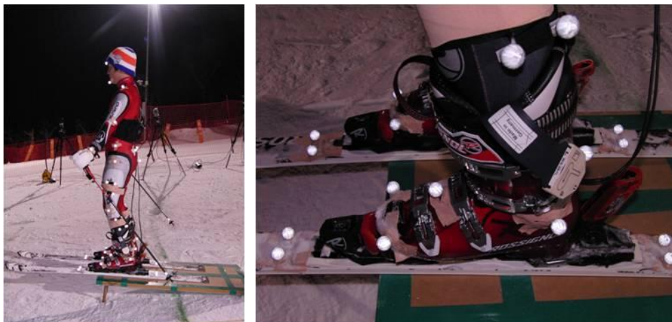
Figure 2: Reflective markers on a skier and marker placements on the boot and the ski plate.
