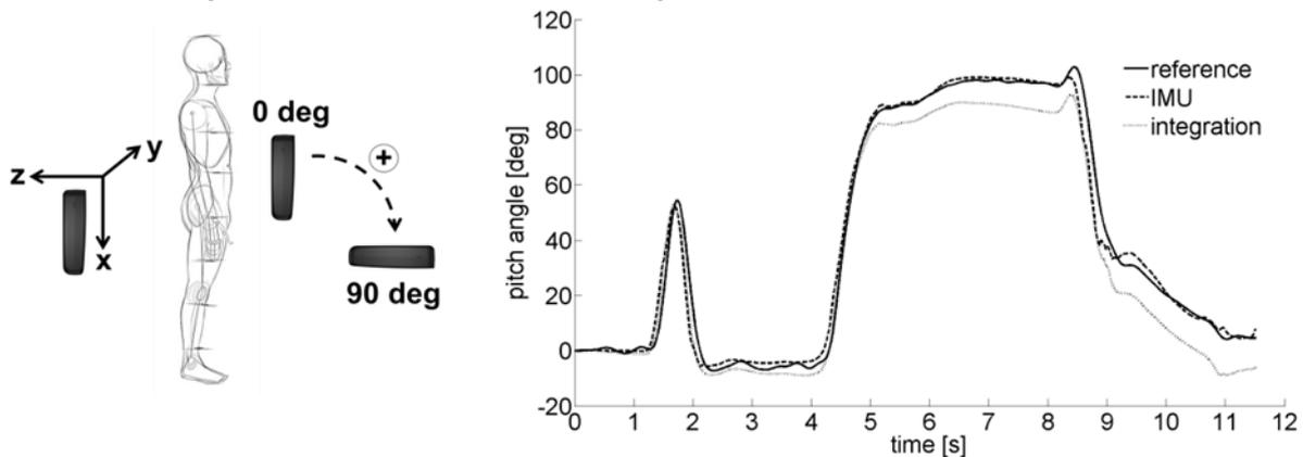
**Figure 1: Pitch angle during the approach phase of the drive block technique for a randomly chosen trial and subject. Reference (solid line), IMU-based (dashed line), and simple integration of the angular velocity (dotted line) estimates are reported.**
