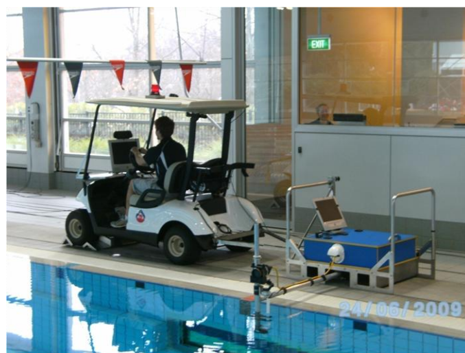
Filming trolley pulled by modified golf cart using two filming cameras (1 above & 1 below water surface).
