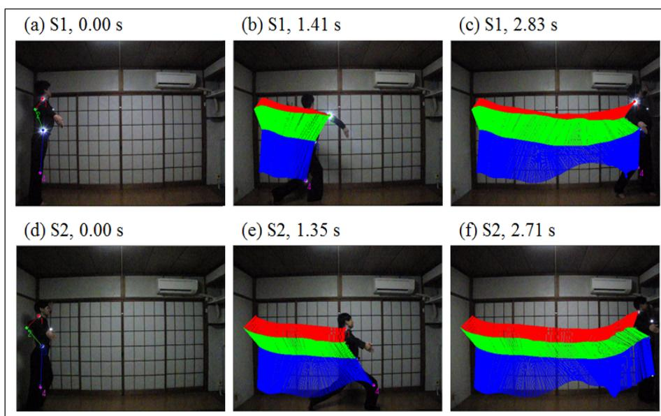
Figure 2: A series of snap shots from the trajectory analysis. (a) to (c) and (d) to (f) show subject 1 (professional license) and subject 2 (amateur license). The neck, elbow, waist, and knee of each subject were illuminated by small LED lights. The position of each LED was drawn as a trajectory. Further, the positions of the neck, elbow, waist, and knee were connected by lines.
