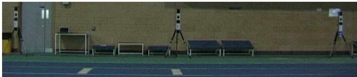
Figure 1: Three CODA CX1 scanners alongside running straight capturing toe marker data at 200 Hz
