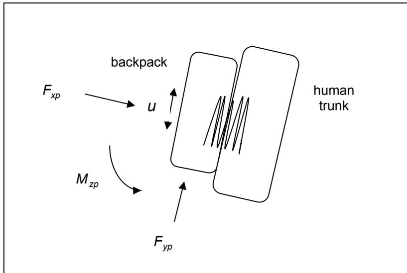
**Figure 1: A free body diagram of a backpack and a human trunk showing the forces exerted on the backpack's centre of mass.**
