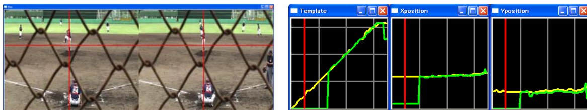
Figure 4: Video window (left) and the transitions of motion category, horizontal position, and vertical position (right). The red line in each transition window denotes current time.
