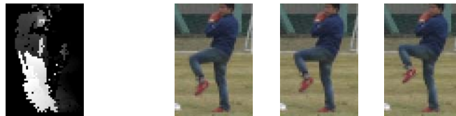
Figure 1: MHI (left) and the snapshots of the corresponding image sequence (right). The motion is raising the left leg.
