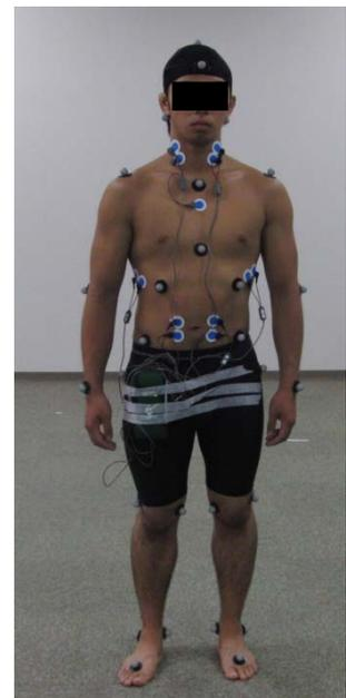
**Figure 2: Placement of reflective markers and EMG electrodes.**
