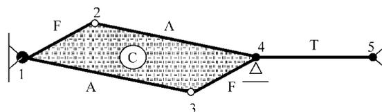
**Figure 4: Mechanical system with elements A, C, F, and T. A, C, and F are not connected in a simplistic way to each other, while T is arranged in series with the complex ACF. C is assumed elastic and incompressible with a shear modulus,  $\mu$ . C plays a sophisticated role in the mechanism of force transmission from F to A to T.**
