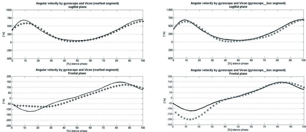
**Figure 2: Representative time-velocity graphs to illustrate comparisons in the sagittal and frontal plane; subject number 1, rearfoot segment: + (left side); gyroscope\_box segment: x (right side); Gyroscope: solid line**
