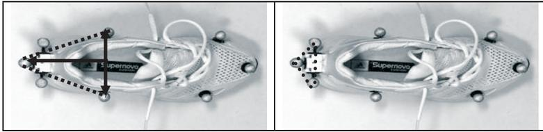
**Figure 1: Marker placement of the shoe model (rearfoot segment: left picture; gyroscope\_box segment: right picture)**
