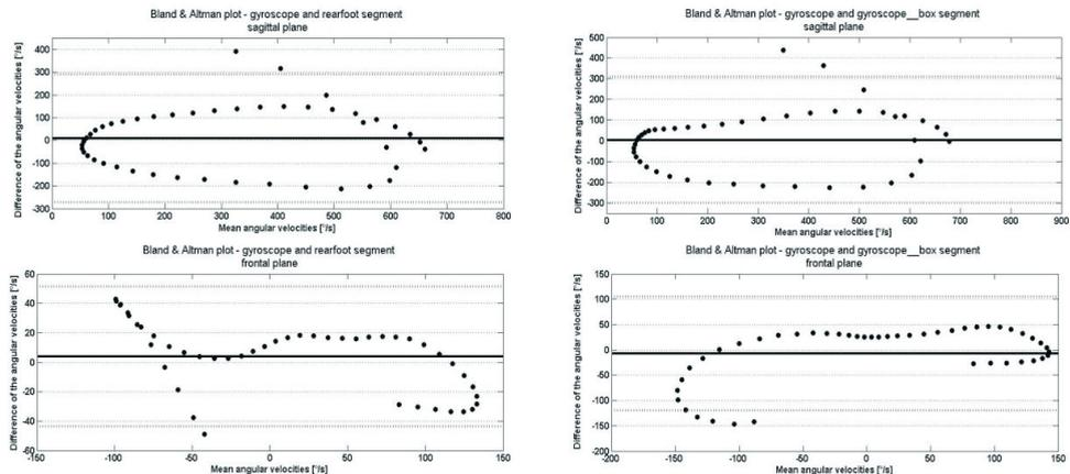
**Figure 4: Bland & Altman plots of the rearfoot segment – gyroscope and gyroscope\_box – gyroscope comparison in the sagittal and frontal plane; subject number 1**
