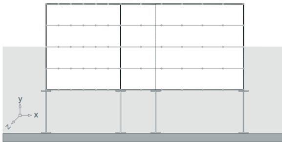
**Figure 2: Calibration volume, with aluminum tubes (black) and steel wires (grey).**
