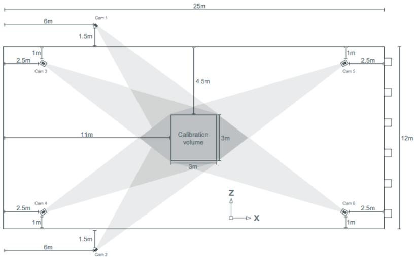
**Figure 1: Upper image of the cameras' field of view in the set up.**
